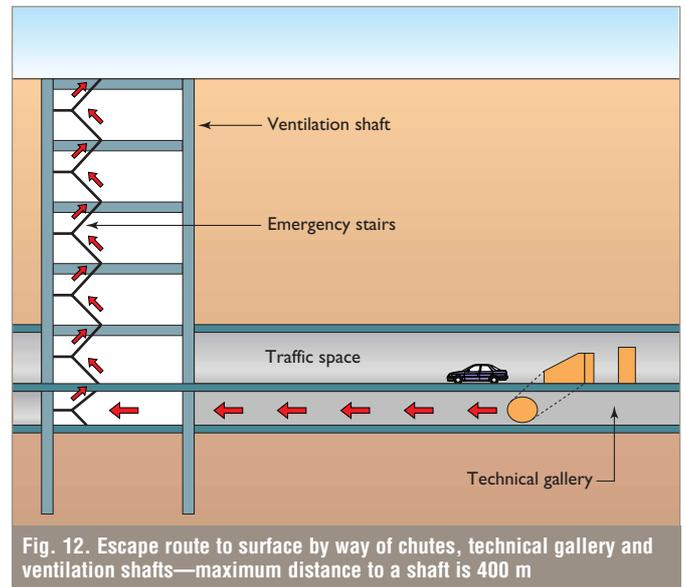
Fig. 12. Escape route to surface by way of chutes, technical gallery and ventilation shafts—maximum distance to a shaft is 400 m
