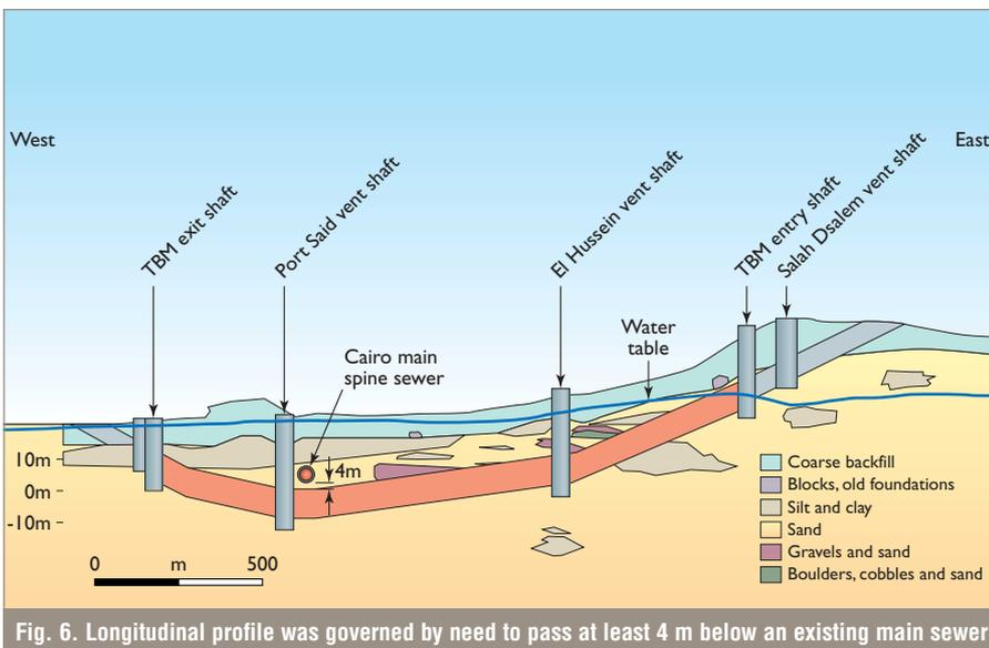
Fig. 6. Longitudinal profile was governed by need to pass at least 4 m below an existing main sewer
