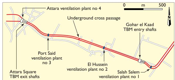
Fig. 3. Final design route for tunnel avoided old flyover piles and resulted in fewer, larger ventilation stations
