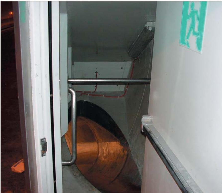
Fig. 14. Entrance to escape chute needs to be kept lit at all times
