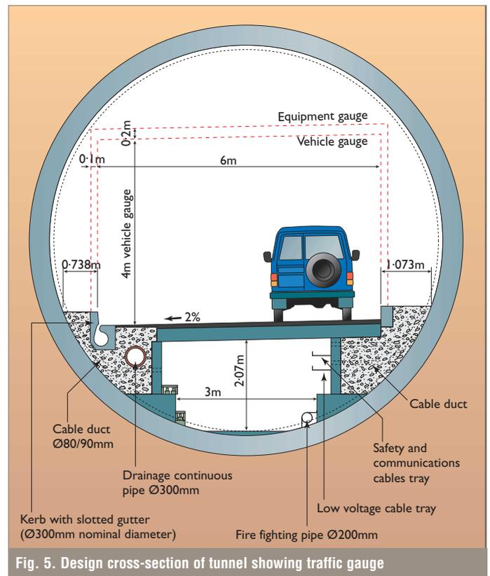
Fig. 5. Design cross-section of tunnel showing traffic gauge
