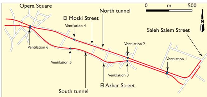
Fig. 2. Concept route for tunnel with north and south bores following main roads
