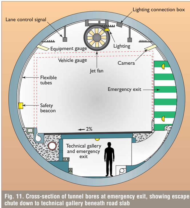
Fig. 11. Cross-section of tunnel bores at emergency exit, showing escape chute down to technical gallery beneath road slab
