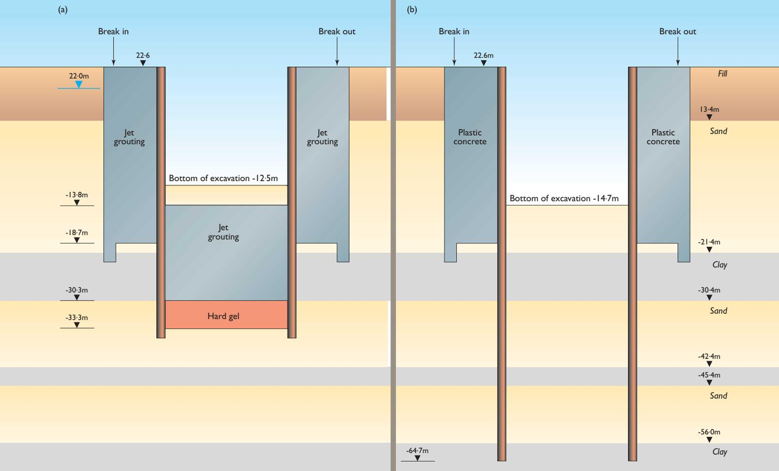
Fig. 4. Original plan for resisting groundwater uplift on ventilation stations involved installing a jet-grouted gel plug between the diaphragm wall (a); whereas the contractor opted to extend the walls down to a watertight clay layer up to 87 m below the surface (b)
